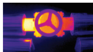
Thermal camera view of the uninsulated valve
