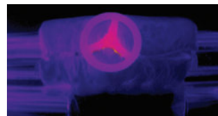
Thermal camera view of the insulated valve after Izocam Valve Jacket application
